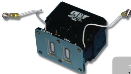
Dual TR Limiter for use in an E-Plane Balanced Hybrid Duplexer. TR tubes are passive, hard brazed tubes. Unit may be manu-factured with optional dummy keep-alive leads. Unit may be supplied phase matched to one or more equivalent single channel units for a monopulse set.
